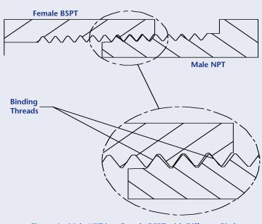
Figure 6 – Male NPT in a Female BSPT with Different Pitch
