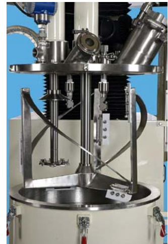
The high speed disperser shaft on this dual-shaft mixer is equipped with a slinger. Helical flights added to the three-wing anchor agitator help improve top-to-bottom mixing.
