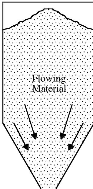
is a first-in last-out flow sequence, with potential caking of stagnant material and sifting segregation in which fines typically exit first. This produces uneven discharge with inconsistent bulk density and uncontrolled flow. As the material level in the vessel drops, layers
