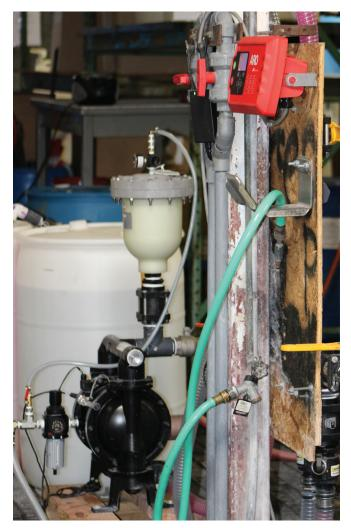
day and reduces the tedium of having to stand and watch the tanks fill to make sure nothing goes wrong. If the Controller senses a problem in pressure or process, it sounds an alarm.
