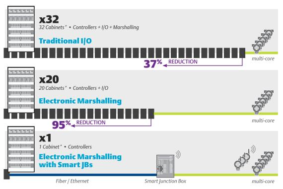
Smart Junction boxes can eliminate \$14M of wiring costs and an additional 95% control room space.
