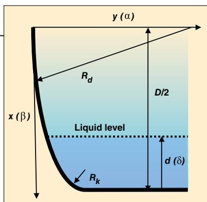
**FIGURE 3.** The coordinate system for a horizontal tank is shown here
