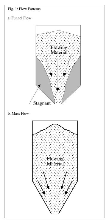
is a first-in last-out flow sequence, with potential caking of stagnant material and sifting segregation in which fines typically exit first. This produces uneven discharge with inconsistent bulk density and uncontrolled flow. As the material level in the vessel drops, layers of the nonflowing material may or may not slide into the following channel. This can produce a stable rathole in the vessel, where material outside the channel remains stagnant.
