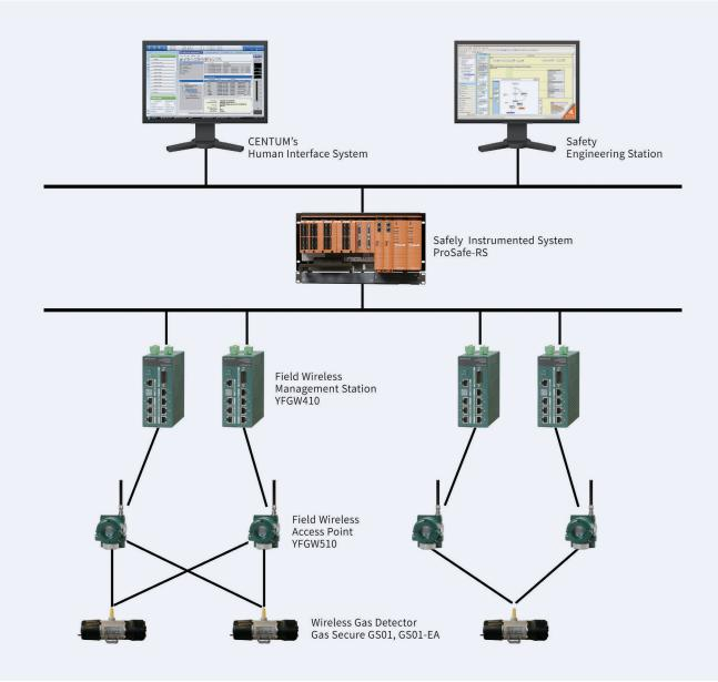
Figure 4 -- Example Yokogawa Safety Instrumented System with HMI and Safety Engineering Station
