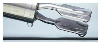
**Figure 2:** The oscillation of a tuning fork instrument changes when a liquid reaches the two forks.
