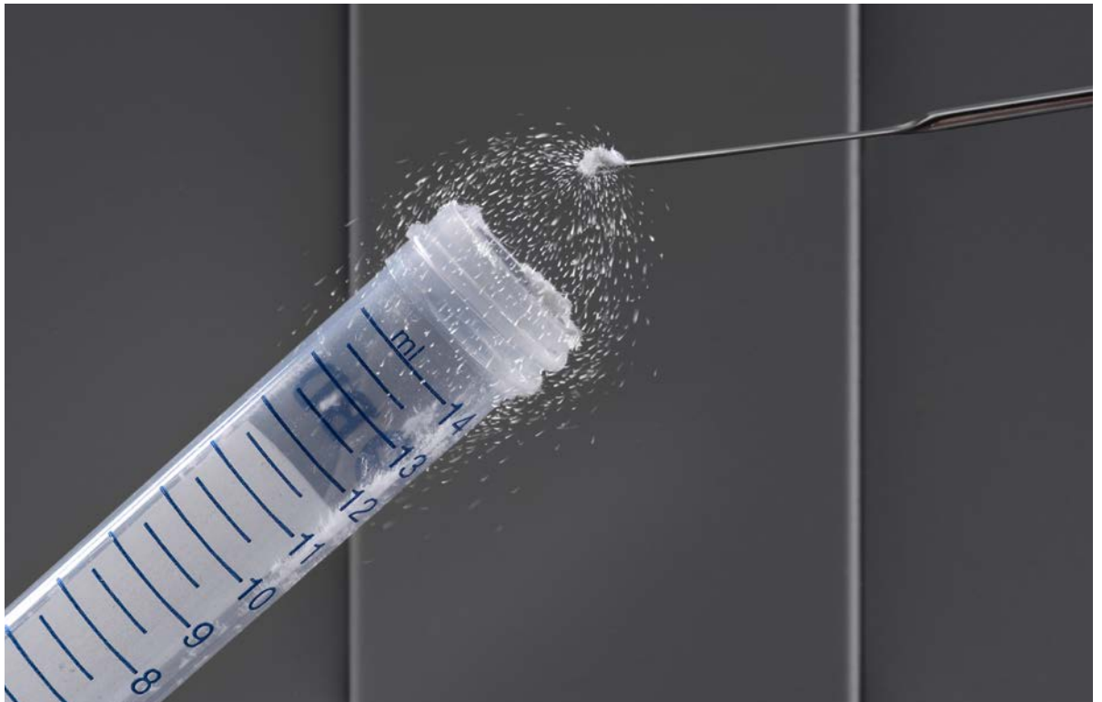
Figure 2: “Jumping” powder during the weighing-in step caused by electrostatic charges.
