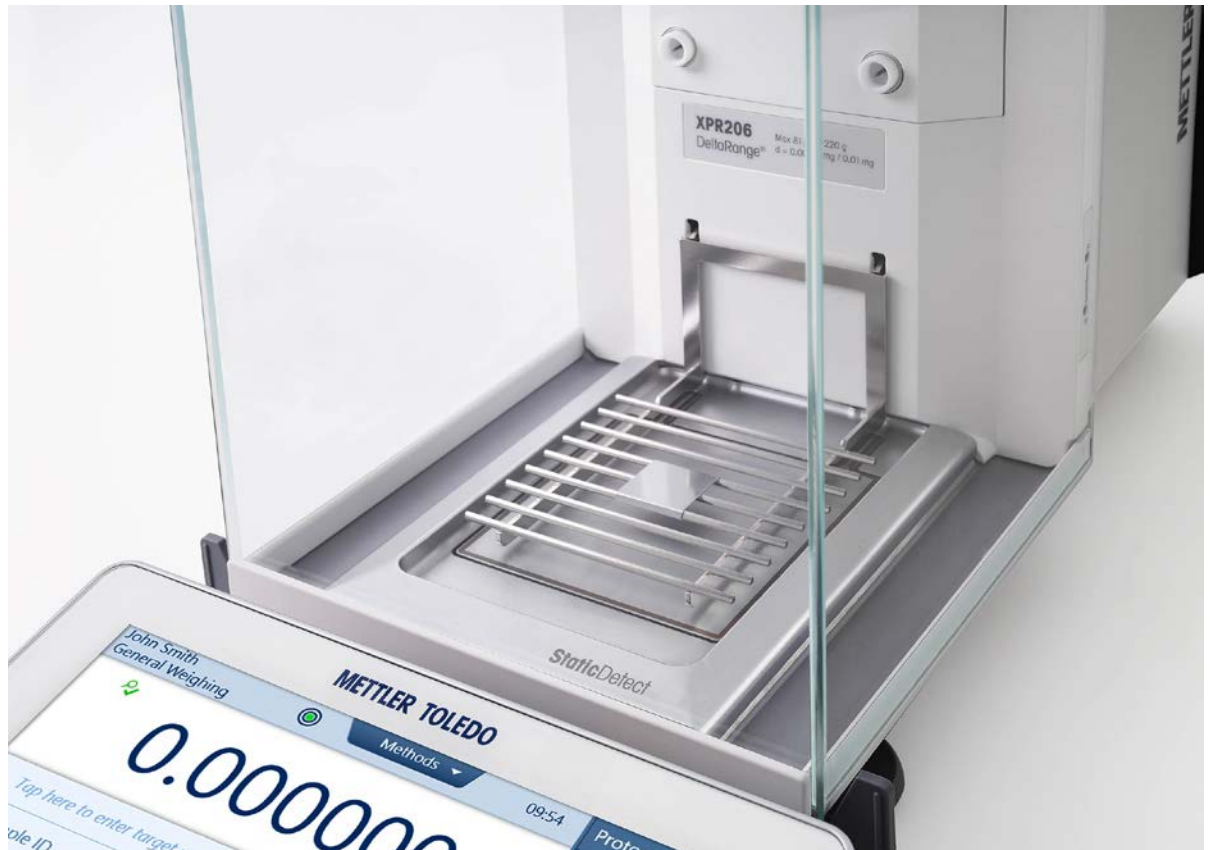
Figure 11: Eliminating static charges with the XPR analytical balance.
