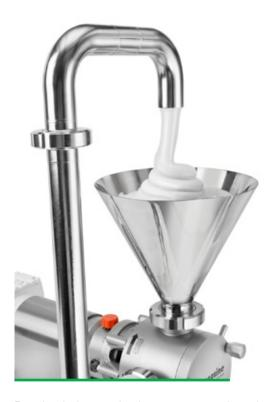
Put simply, if a production or process plant changes to a higher viscosity product, the impact on a sine pump if minimal if not negligible. For instance, using the same application parameters as before, but switching from a 20,000 cP product to a 200,000 cP product, the VHP of a sine pump increases by around 0.1, to 0.3 VHP (0.22 kW).
