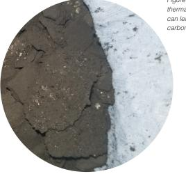
Figure 2: Excessive thermal degradation can lead to hard carbon deposits.
