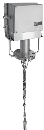
Figure 6: Multiple thermocouple or RTD sensors fitted to a metal rope, and connected to a multipoint temperature transmitter, can be used to monitor the temperature profile within a vessel.
