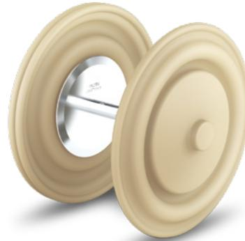
*The new Chem-Fuse Integral Piston Diaphragm (IPD) from Wilden® reduces the risk that damaging product buildup will occur in AODD pumps through a design that encases the diaphragm’s outer piston within the diaphragm material itself.*
