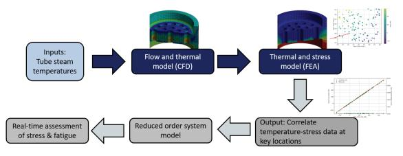
Figure 5. Building a process for heat exchange integrity.
